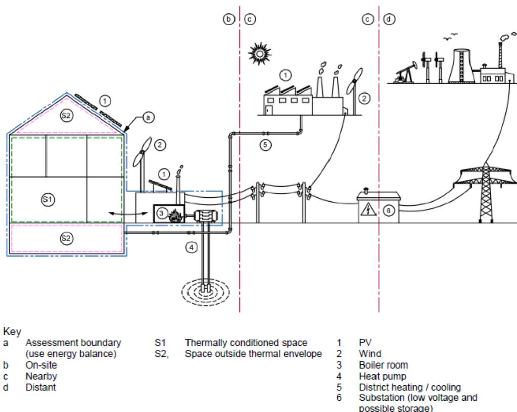
Figure 1.1.1 Building assessment boundary and energy balance locations
